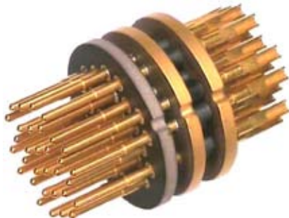
Fig. 6 The internal configuration of a varistor protected unbalanced Pi
