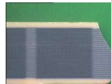
Tandem Capacitor Post bend and life Test - Cap loss Approx. 50% NB - Capacitor still Functioning
