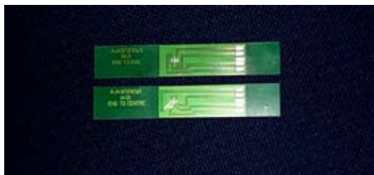
Example of FR4 Test PCB Used
