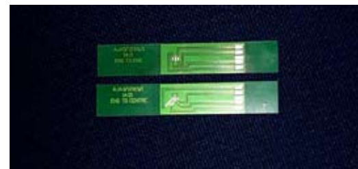
Example of FR4 Test PCB Used
